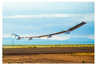
Japanese telecommunications company SoftBank Corp. is developing a solar-powered aircraft. PHOTO: SOFTBANK CORP.
